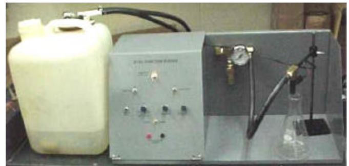
Figure 6 - Fuel injector test stand
